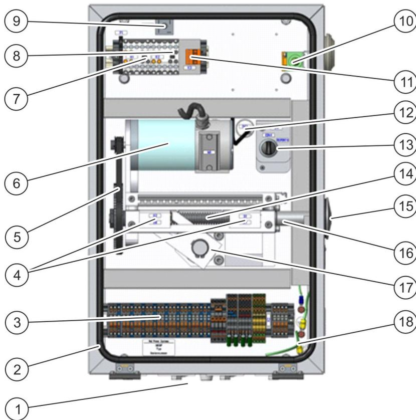
Fig. 2: Overview of TracFeed® SFA inside
