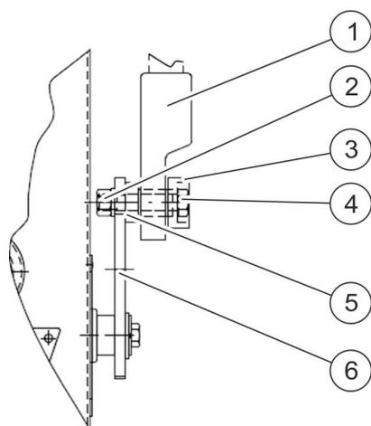
1. → Secure the lower section of the shift linkage (Fig. 15/1) onto the retaining bolt (Fig. 15/5) with a locking ring (Fig. 15/3). Secure the bolt (Fig. 15/4) with a nut (Fig. 15/2) (tightening torque 50 Nm).
