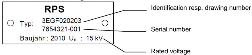
Serial number of the remote motor drive is located on the right-hand side of the enclosure:
