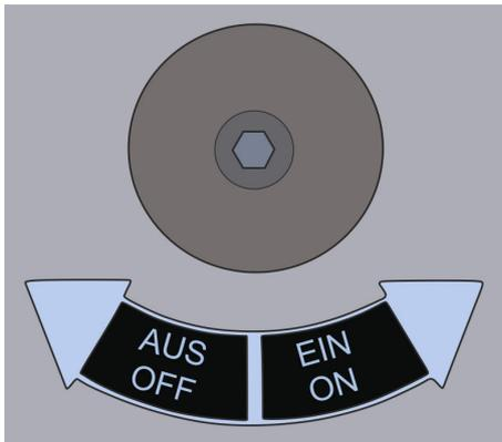
Fig. 8: Labelling of the cranking direction
