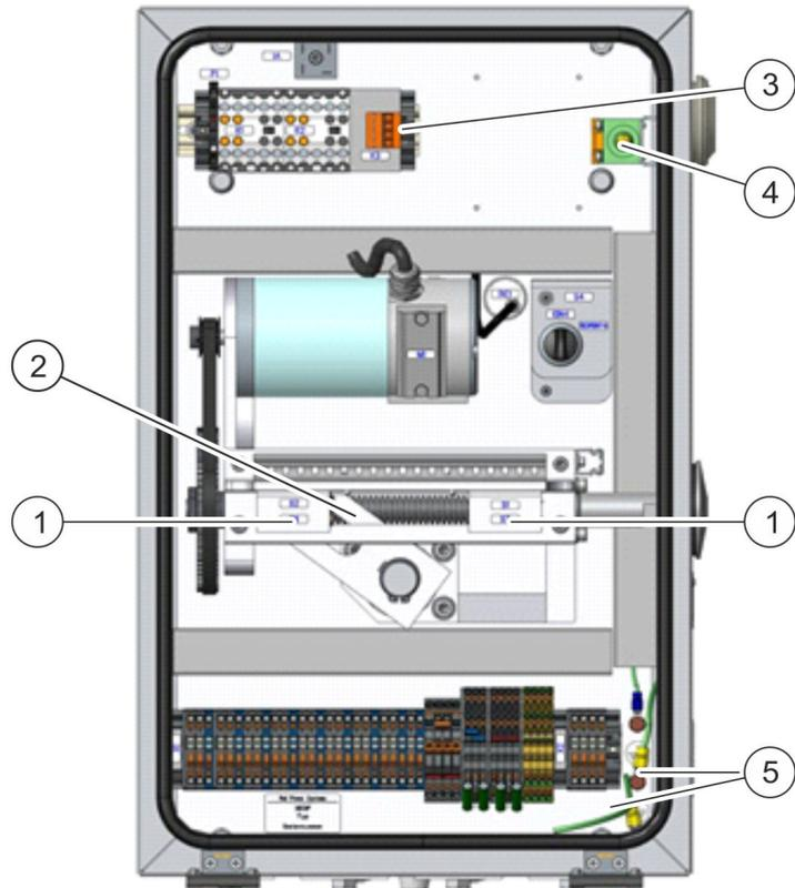
Fig. 3: Location of the safety devices
