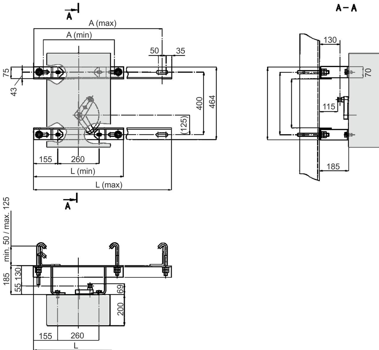
Fig. 11: Examples for assembling the TracFeed® SFA on a lattice steel mast or flat-frame mast
