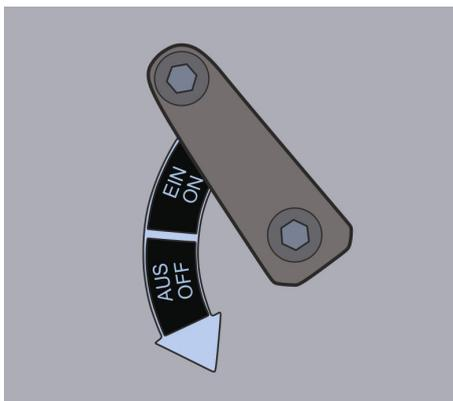
Fig. 9: Labeling of the switch stroke
